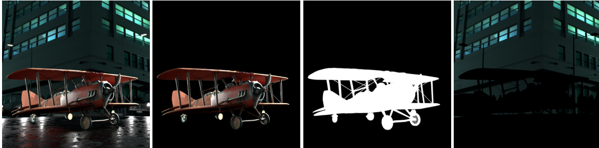
Figure 1: Any object can be isolated with a perfect antialiasing from a single OpenEXR/Id file: everything, the plane alone, the mask of the plane, the buildings. All images ©2015 LPPTV - LITTLE PRINCESS - ON ENTERTAINMENT - ORANGE STUDIO - M6 FILMS - LUCKY RED
